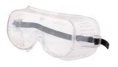
Goggles with soft PVC frame and 13-mm long black adjustable rubber band. Clear polycarbonate lens 1,5 mm thick are resistant to medium-energy shocks (up to 120 m/s) at extreme temperatures (-5°C - +55°C). Top-quality goggles provide maximum protection and comfort because of direct aeration system which protects against fogging and provides protection against liquid drops, molten metal and hot solid substances. It can be used separately or over dioptric glasses.
